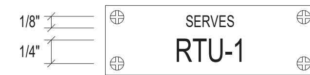
SWITCHBOARD/DISTRIBUTION PANEL/MOTOR CONTROL CENTER BREAKER/SWITCH
